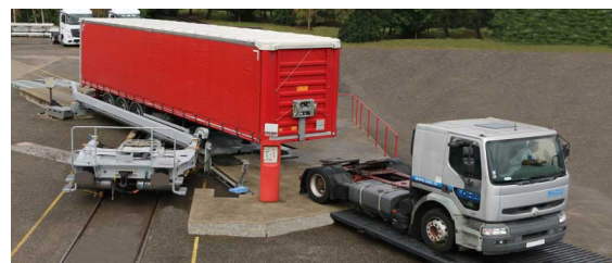
New technology in Europe allows rapid transfer between road and rail, increasing overall efficiency for freight movement
